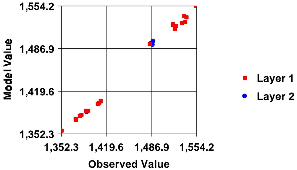
Figure 30 - Observed vs. Computed target values for the steady-state calibration.
