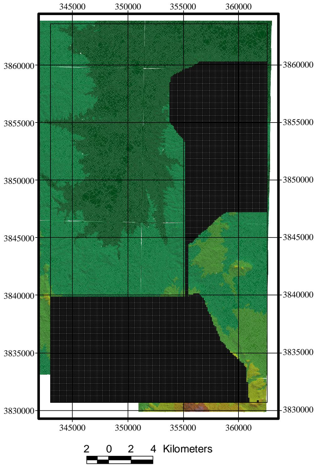
Figure 21 - Triangular Irregular Network (TIN) of the MWWVS overlain by the active and inactive model area. Coordinate grid is UTM Northing and Easting.
