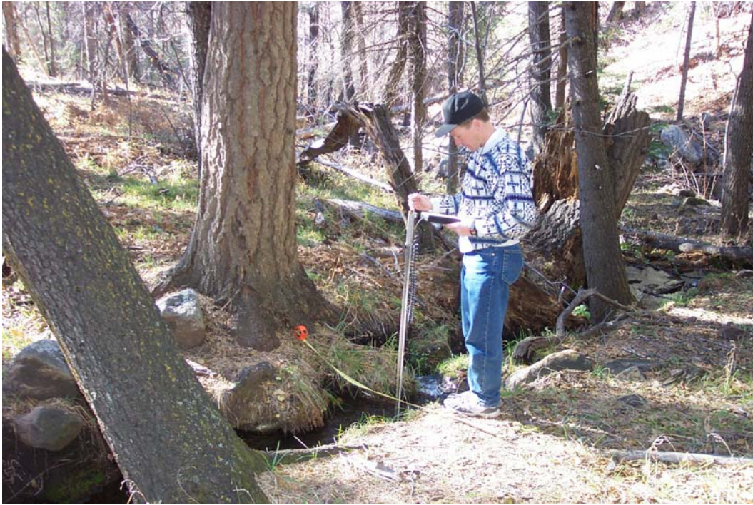
Figure 14 – Rheocrene spring using a flow meter to measure discharge in the spring channel (Pieper Hatchery Spring, Abe Springer pictured 12/12/02).
