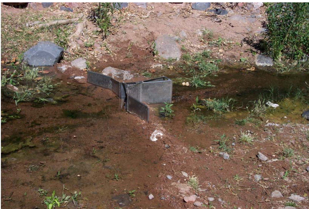
Figure 16 – Limnocrene spring flow measured in spring channel using the box flume (LX Spring 6/13/02).
