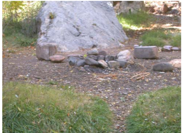
Floodplain Condition and material at Cross-Section #4 Sta: 9+25. Floodplain ( n=0.085 )
