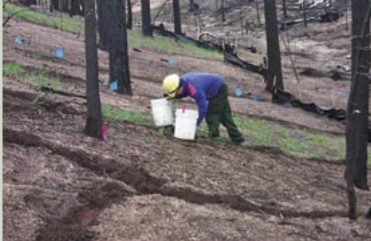
Measuring ground cover on treated hillslope plots; silt fence in background.
